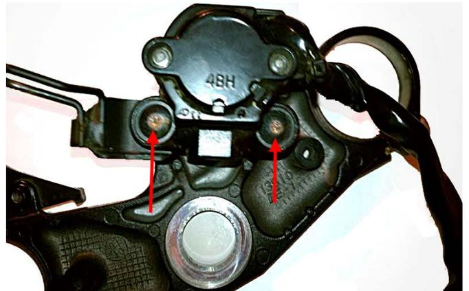
4. Reinstall the top triple clamp. NOTE: to reinstall the key switch at a later date, remove the studs from the underside of the clamp and replace them with regular bolts. To make these connections secure, use button head allen bolts for installation and then drill the hex out so that it is round.
